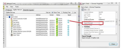
Be aware that the signal strength is only the strength the ZigBee device has to its *first* routing node. For this reason, it is important to use the *Routing Tree* to look for ZigBee devices with weak signals that other ZigBee devices may route through back to the ZAP.
