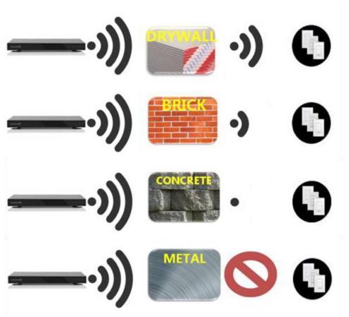
• Another example of how different building materials can affect 2.4 GHz signals can be found <a href="here">here</a> (information on 2.4 GHz signal attenuation caused by common building materials from the City of Cumberland, MD website).
