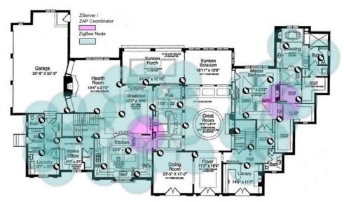
Following is an example of a multiple ZServer/ZAP (multiple ZigBee mesh) system.
