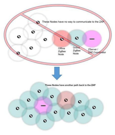
Locating your ZAP in a central location will give greater routing flexibility in the event that a ZigBee device falls offline.
