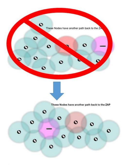
**NOTE**: The images above are not the full mesh; rather, a section of a larger mesh that shows how nodes would have another path to a ZAP.
