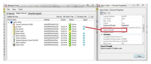
• On the same page, you can also enable an LED blink that will make the LEDs on the newer-generation ZigBee devices blink a color that indicates the signal strength (Green = good, Yellow = fair, Red = poor).
