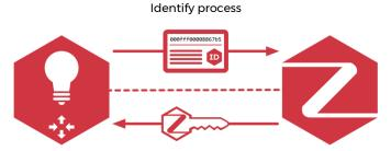
The Zigbee device sends its ID to the mesh controller, and the mesh controller sends the mesh's security key to the device.
