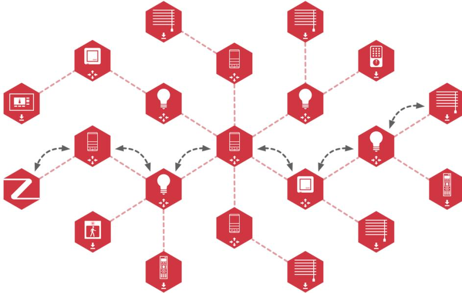
When the mesh controller is centrally located, performance improves because there are fewer hops to each device in the mesh.
