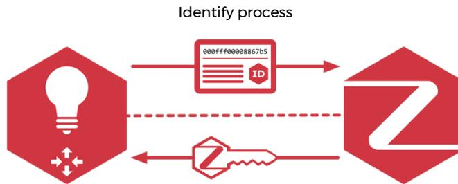
The Zigbee device sends its ID to the mesh controller, and the mesh controller sends the mesh's security key to the device.
