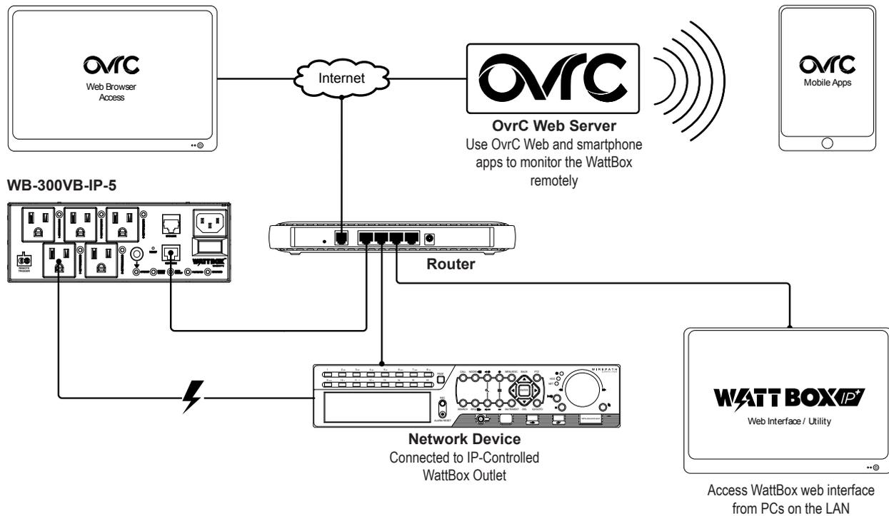
Connect the WattBox™ and any equipment monitored and powered by the WattBox to the local network as illustrated.
