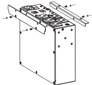
2. Open the knockout in the bottom of the VersaBox and install the enclosure. Insert the WattBox after the enclosure is installed.
