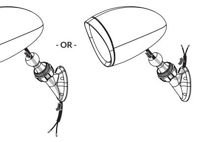
Slide the collet nut up to the enclosure and lightly tighten in
