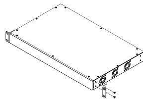
**Note:** Rack ears can be installed to the front or the back of the amplifier as needed.
