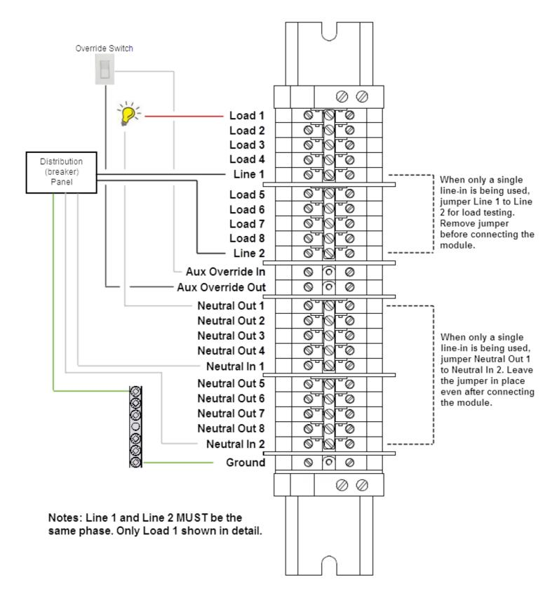
Figure 2. 8-Channel Dimmer Terminal Block Wiring
