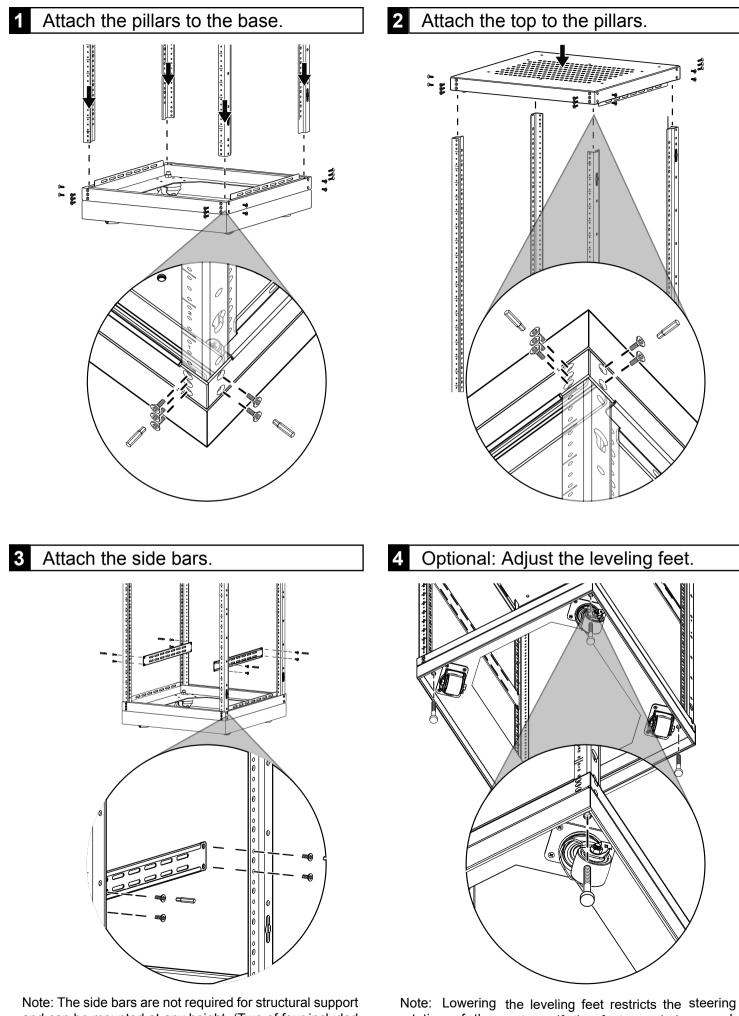
Note: The side bars are not required for structural support and can be mounted at any height. (Two of four included bars are pictured.) Note: Lowering the leveling feet restricts the steering rotation of the casters. If the feet are being used, position the rack before installing equipment.
