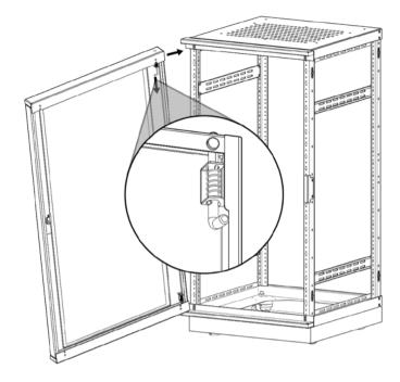
Note: Before installing the door, position the hinge bushings in the holes on the top and bottom brackets on the side that swings.
