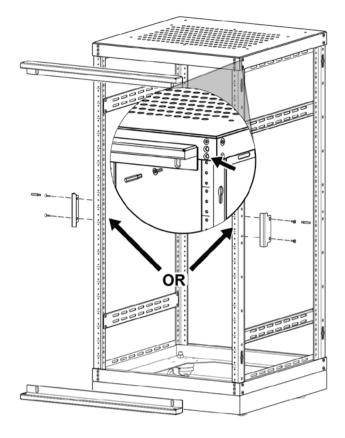
Note: The door may be installed for left- or right-hand swing. The hinge brackets are held on by 1 screw in each corner. The brackets are also slotted so that they can be adjusted for optimal door fit.
