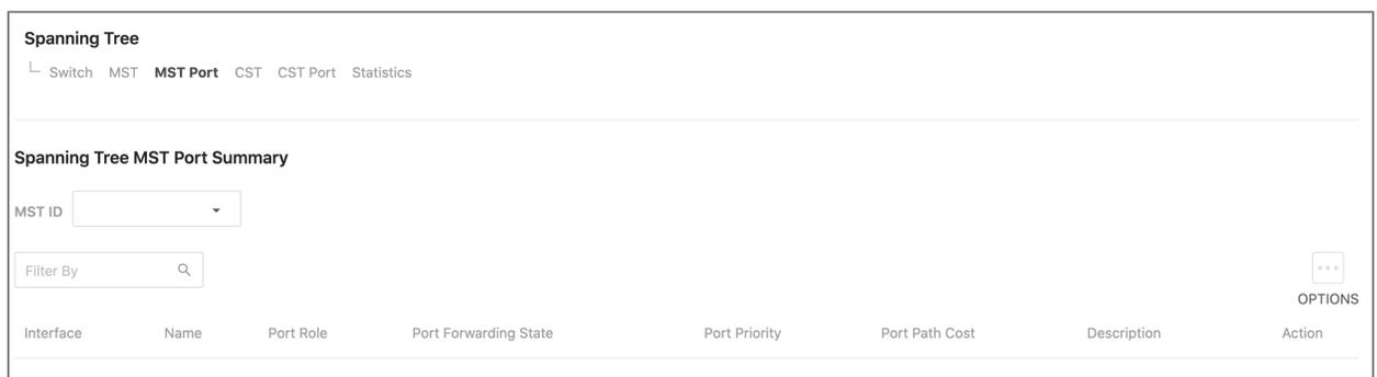
An MST instance must first be created under the *MST* tab before an MST ID can be selected. Once selected, all ports are shown, can be configured, and more detail can be viewed by selecting **Edit** for the desired interface.
