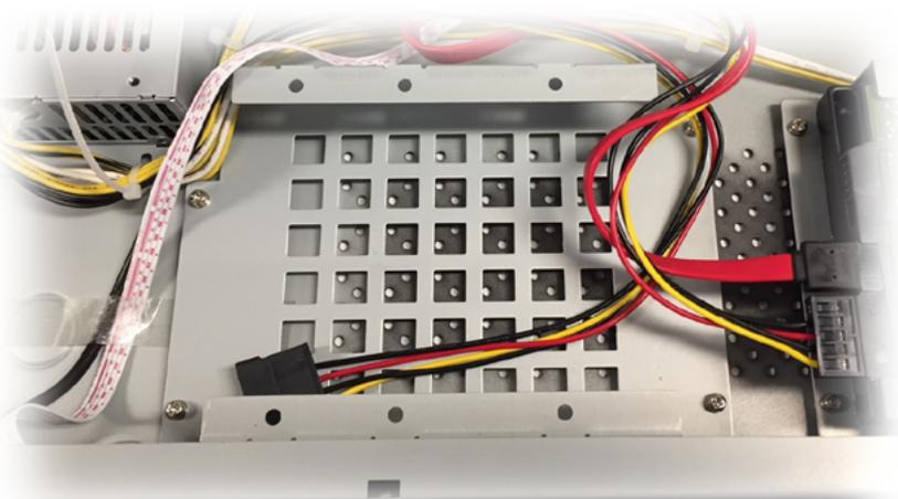
Insert four screws (as shown below) to hold the hard drive in place.
