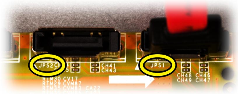
Be sure to connect them in the correct order. Looking at the recorder from the front of the unit, the SATA ports are numbered 1 and 2. Looking closely at the board, you can actually read the numbers beside each port after the letters *JPS*.
