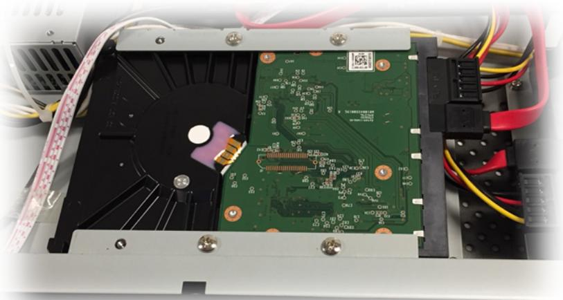
Remove the four screws that hold the hard drive in place and carefully slide the hard drive out.
