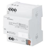
KNX power supplies generate and monitor the KNX system voltage (SELV). The bus line is decoupled from the power supply by an integrated choke.
