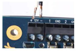
No power jumpers or settings are required—connect one or the other (line power or external DC power supply).
