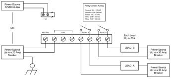
Option 3: Applicable where a combination of power sources are used; load "A" is powered by an external breaker in the load path, and load "B" is powered by the device's external breaker or power source:
