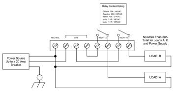
Option 2: Applicable where each load uses its own external circuit breaker:
