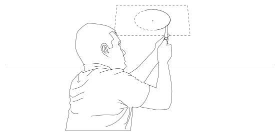
4. Fit the bracket into the opening and ensure it sits flat against the drywall.
