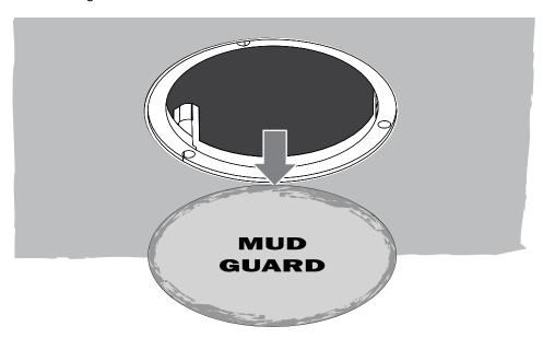
**Pro Tip:** Ensure there is no mud on the inner lip of the bracket. Mud in this area will affect proper speaker mounting.
