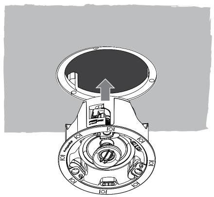
11. Install a round frameless grille (SKU: ESS-GLXRND-IC-X), which attaches magnetically to the speaker.
