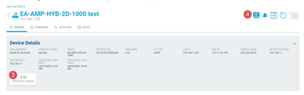
5. Once the update completes and the hybrid amplifier is online in OvrC again, click the device name and confirm the firmware version once more.
