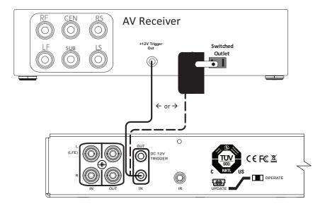
If the receiver does not have a 12V trigger output, using a 12V power supply plugged into a switched outlet on the receiver provides the same functionality. Connect the appropriate conductor to each screw terminal, observing correct polarity.
