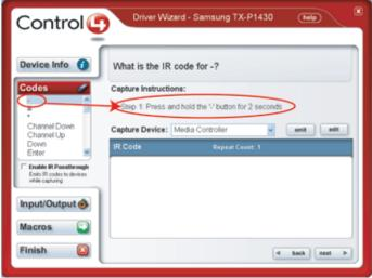
When a code has been captured, Composer Pro puts a check next to the captured code in the Codes list, and selects the next code to be captured. When you capture all the codes, Driver Wizard automatically moves you to the next section: 'Input/Output.'
