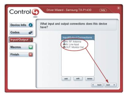
18 When the Input/Output Connections list is completed, click next.
