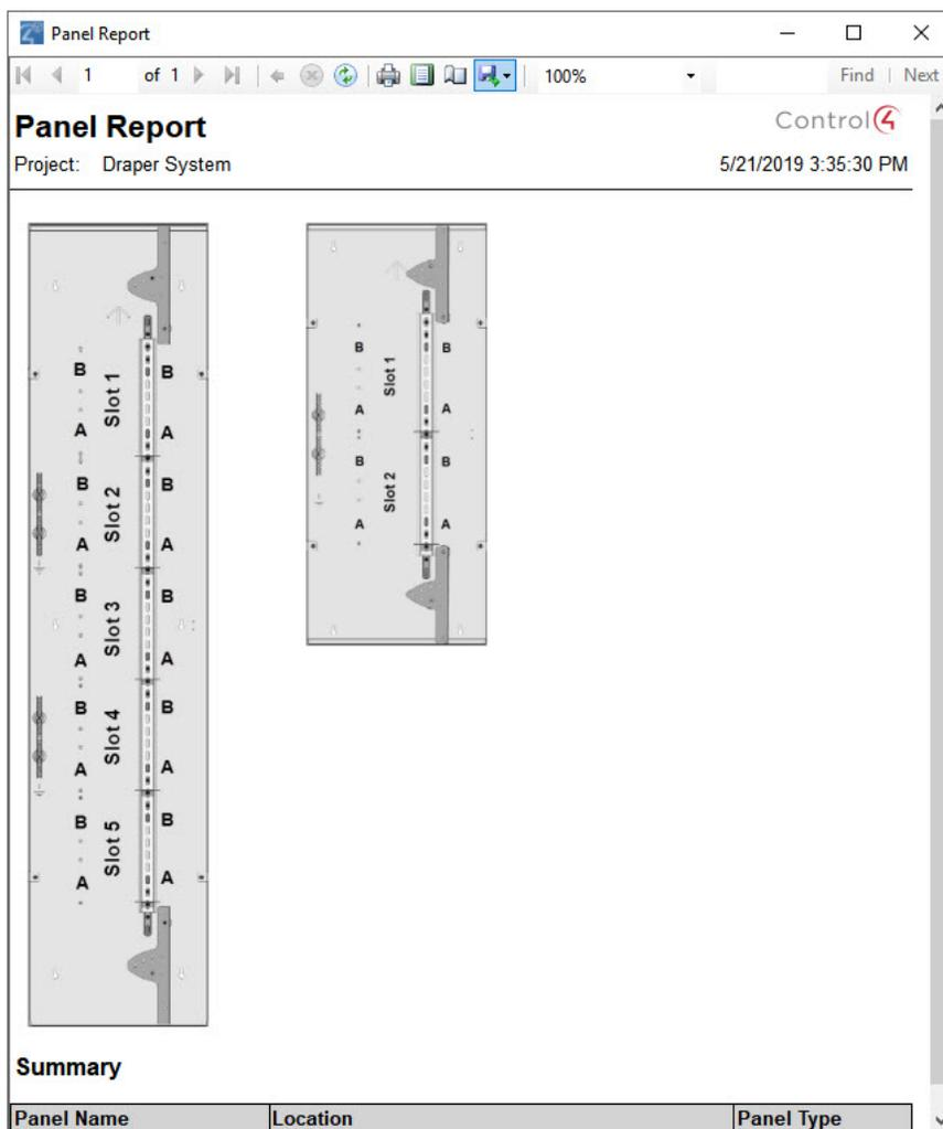
3. View, save, or print out the report. The report shows a graphical view of the panels and where the devices should be installed.
