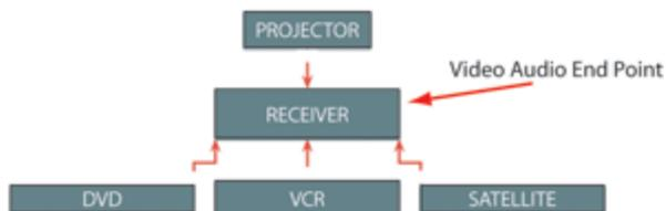
Example 5: **Audio End-Point**—The receiver switches audio for DVD, VCR, and satellite.
