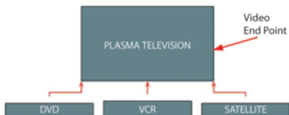
Example 4: **Video Audio End-Point (combined)**—The receiver switches both audio and video for DVD, VCR, and satellite.
