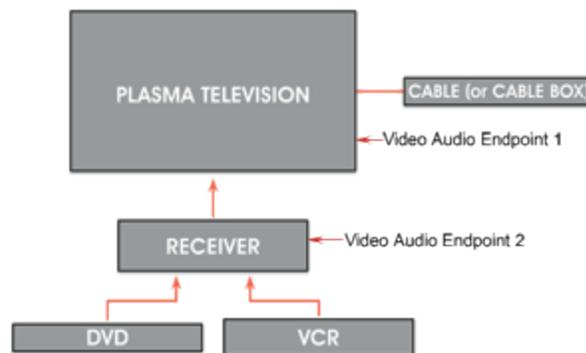
Example 2: **Video Audio End-Point 1**—The receiver is Video Audio End Point 1 and manages the volume in the room when the homeowner watches video using the DVD, VCR, or cable.
