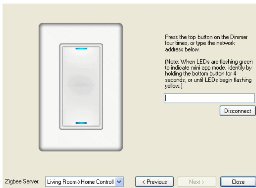
5. When the Light Switch identification screen appears, press the **top** button four times. When the address appears, click **Next**.
