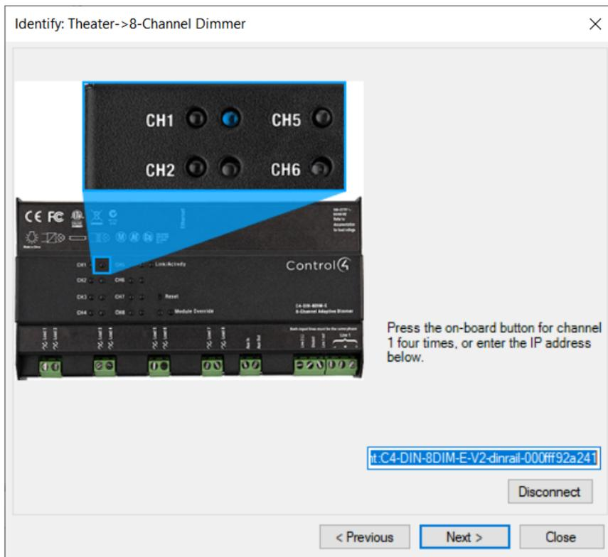
4. Select **Dimmer**, and then click **Identify**. The screen to identify the dimmer appears. Press the top dimmer button **four** times. This identifies this specific dimmer with a
