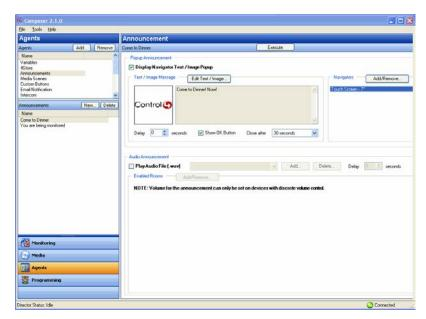
8 Audio file. Add a **WAV** audio file and set up the audio file to play (see the figure below).
