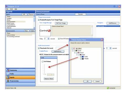
**Note:** Volume for the announcement can be set only on devices with discrete volume control.
