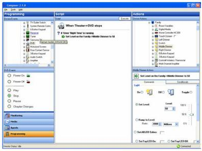
All programming is based on events and actions in a Control4 system. For example, if a door opens, it is an *event*. When an event occurs in the system, it can trigger programmed *actions* to take place. For example, when the bathroom door opens (event), you can program the bathroom light to turn on (action).
