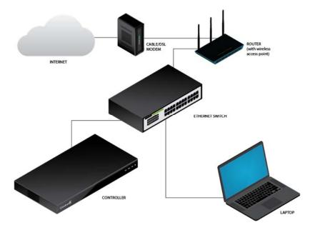
The *router* is the heart of your home computer network. It uses a *modem* to communicate with the Internet. The router provides wifi that wireless devices (such as laptops and smart phones) can use to connect to the network and the Internet. The *switch* provides additional wired connections to the home network.
