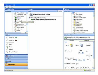
All programming is based on events and actions in a Control4 system. For example, if a door with a sensor opens, it is logged as an *event*. When an event occurs in the system, it can trigger programmed *actions* to take place. For example, when the bathroom door opens (event), you can program the bathroom light to turn on (action).
