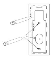
**Important!** The VDB should never be mounted more than 6 ft (2 m) off the ground.
