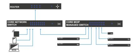
**Note:** If there are physical limitations that do not allow you to connect your Core MoIP switch to your Core Network switch you can connect the Core MoIP switch to an Edge Network switch, but we highly recommend keeping the Core MoIP switch connected to your Core Network switch when possible.
