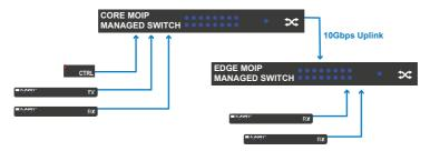
If you're sharing a switch between MoIP and non-MoIP devices, follow the VLAN rules outlined in the Advanced Configuration section.
