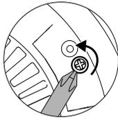
2. Disengage the dog ears on the bracket. Use a #2 Phillips head screwdriver to push the dog ear back and turn it counter-clockwise.
