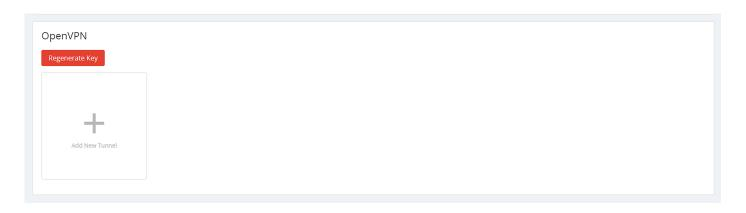
Click the **+ Add New Tunnel** button and enter the name of the VPN as well as the server IP address, which is typically the same as your WAN IP address for the router. If a DDNS connection is active, use the first DDNS entry. Only change this field if a different DDNS service or static IP is being configured on the WAN side.
