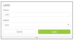
Click on a port to open a dialog where you can change the LAN's name, speed settings, and duplex setting (if the port is not set to auto). This also shows the actual speed at bottom, color coded as normal.
