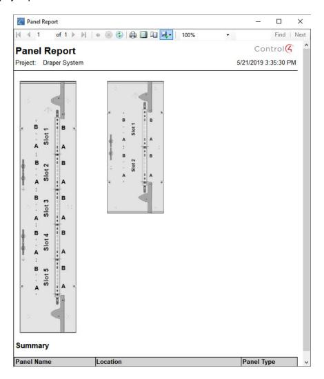
3. View, save, or print out the report. The report shows a graphical view of the panels and where the devices should be installed.
