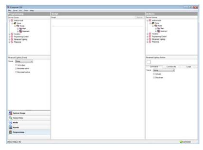
A programming example for use with the Advanced Lighting agent might be in a case where, if the front door opens and it's past 9 PM at night, all the lights turn on in the home at various levels.
