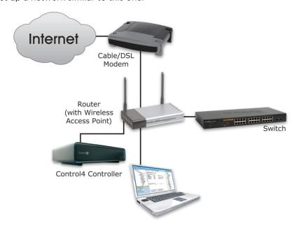
The *router* is the heart of your home computer network. It uses a *modem* to communicate with the Internet. The router provides wifi that wireless devices (such as laptops and smart phones) can use to connect to the network and the Internet. The *switch* provides additional wired connections to the home network.
