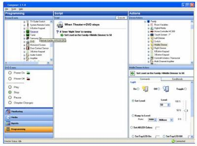
All programming is based on events and actions in a Control4 system. For example, if a door opens, it is known as an *event*. When an event occurs in the system, it can trigger programmed *actions* to take place. For example, when the bathroom door opens (event), you can program the bathroom light to turn on (action).
