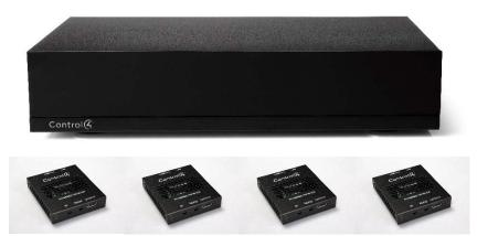
Interconnection between the matrix switch and associated HDBaseT receivers is through one single CAT5e, CAT6, or CAT7 cable for each zone. Single CAT5e/6/7 cable interconnect between these components is made possible by the use of HDBaseT technology. HDBaseT enables video and audio, as well as power, Ethernet, IR, and RS-232 to all be sent over large distances by a single cable per zone.
